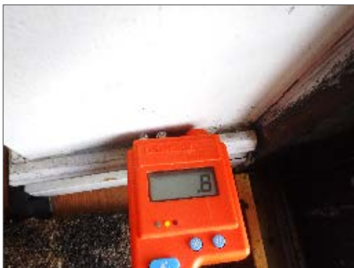
Photo 3 – Wet wall finishes identified in Unit 102.
